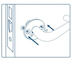
Mount the inner handle set and tighten all fixing screws fully.
