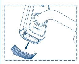
Remove the outer battery cover.
