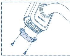
2 Remove two screws and inner battery cover.
