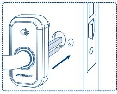
2 Push the stud and spindle through the door.
