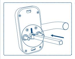
Make sure the spindle is pushed all the way into the lever with right position.
