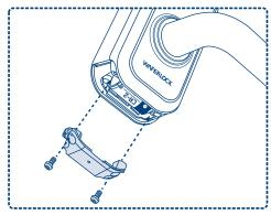
4 Attach the inner battery cover and tighten the two screws fully.
