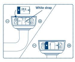
Insert CR2 battery and make sure the white battery strap is properly under/cross the battery. (It helps you remove the battery easily).
